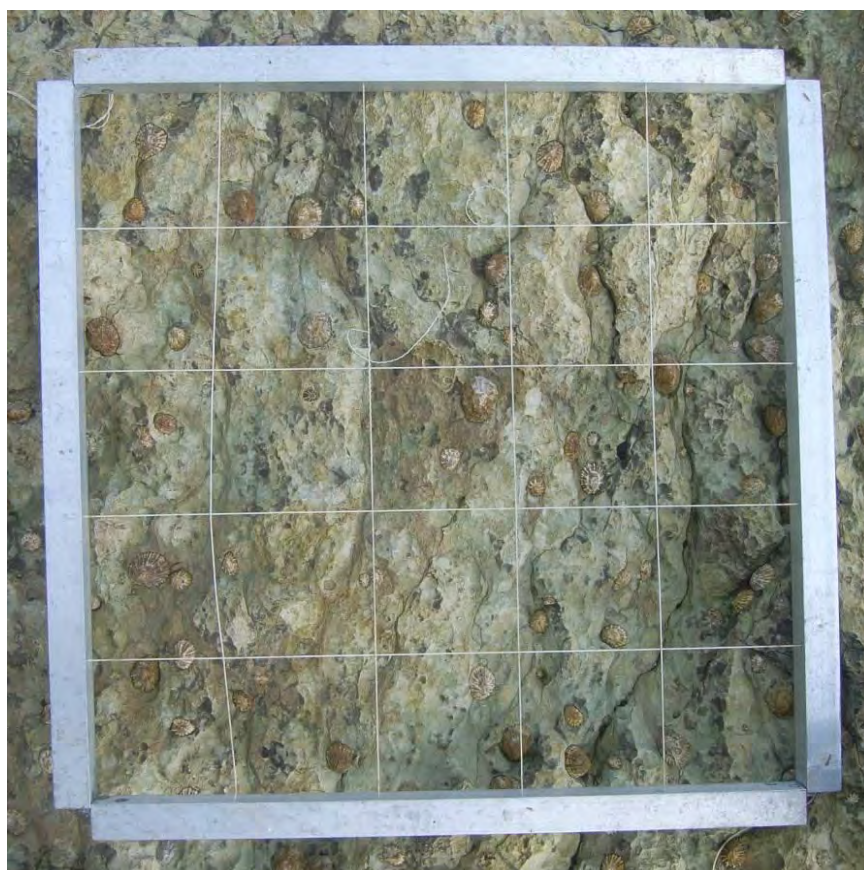
Figure 3. MarClim 0.25 m 2 limpet quadrat used for surveys.
