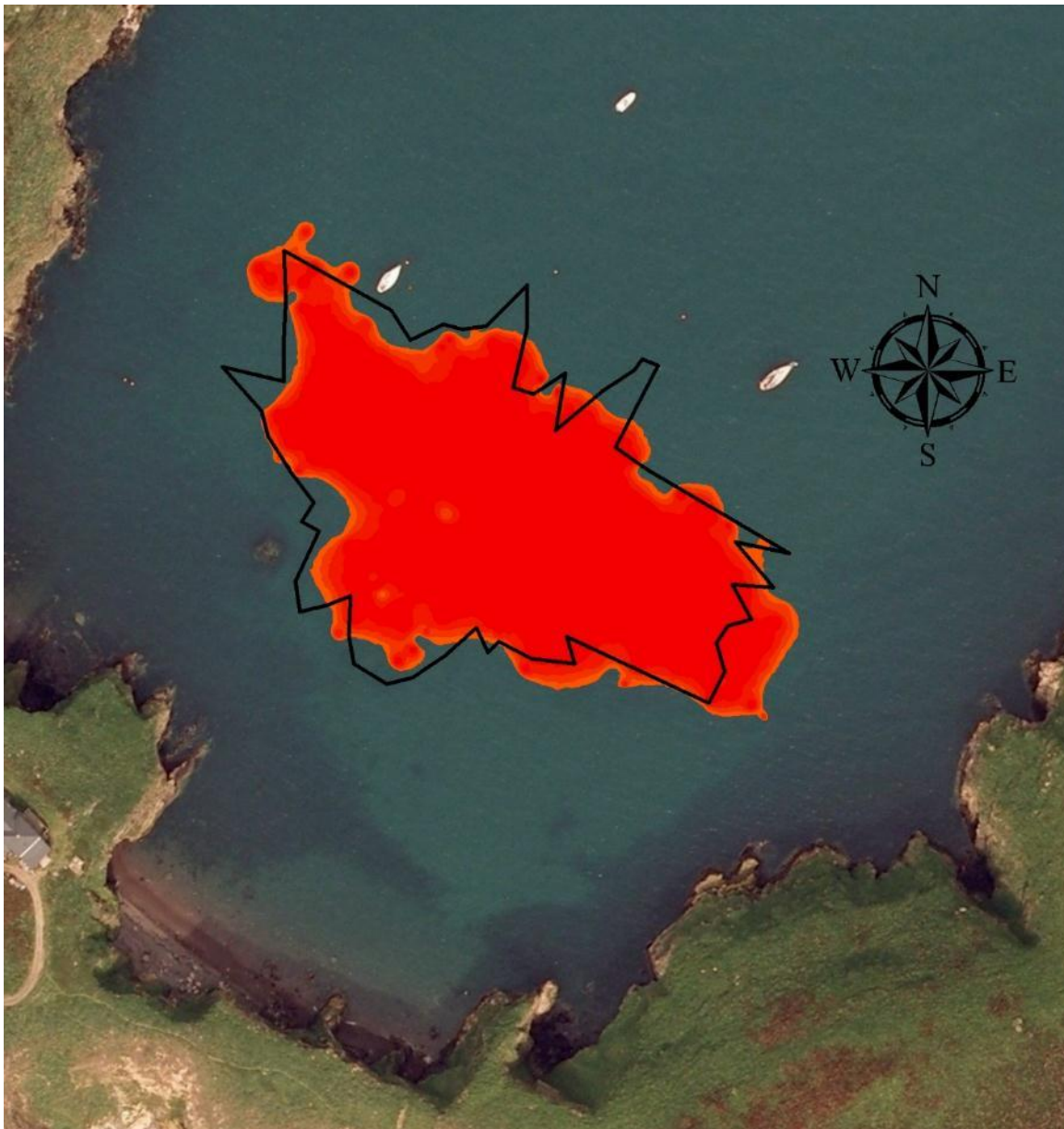
2014 Boundary Polygon (black) overlaid onto the 60% %AI contour boundary from the 2014 Acoustic survey.
