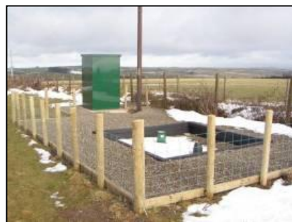
Figure 5– new telemetry rain gauge used to record rainfall in real time at Rhos Ymyrson in the Teifi catchment.
